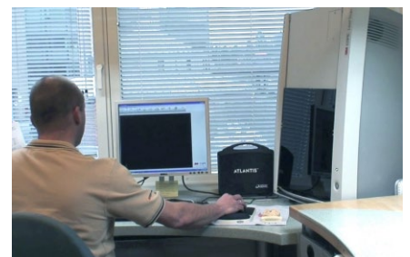
27. The model is scanned in the 3M ESPE Lava scanner and the files are sent to the DENTSPLY Implants ATLANTIS production unit where an individually designed abutment will be manufactured.
